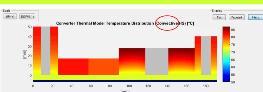
Same DC-DC Converter Design and problem specifications as in GUI (left), but different heat dissipation at heatsink.
