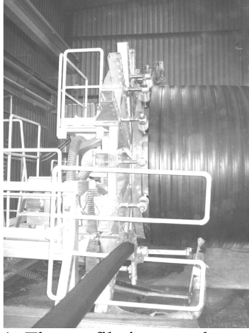
Figure 1: The profile is wound around a mandrel and welded to the adjacent one.
