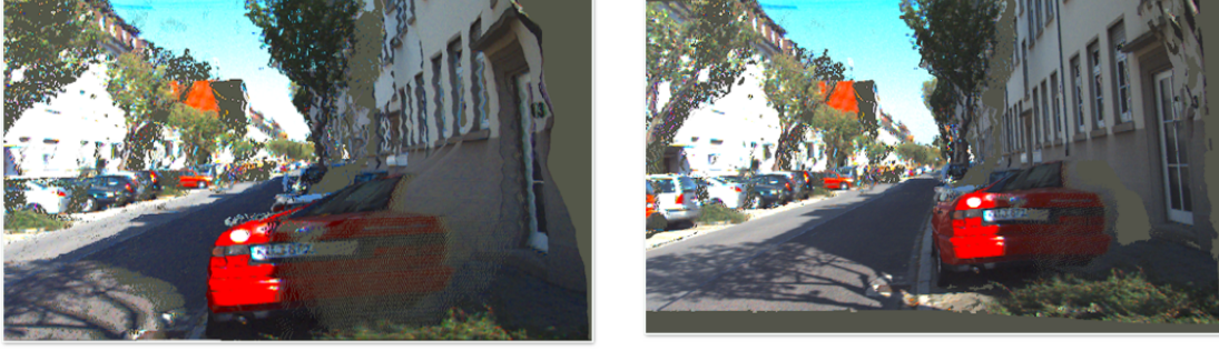
Fig. 1. A qualitative perspective of this paper. A dense depth-map (left) of a planar wall surface created by a state-of-the-art Total Generalised Variation algorithm is displayed. As expected the algorithm results in a noisy output on the largely textureless wall and road. Explicitly discovering planar regions and from there invoking a planar prior to restricted areas results in an improved depth-map (right), showing a marked improvement in the depth estimation along the wall and road.
