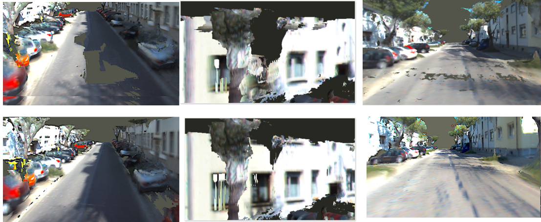
Fig. 2. Sample results of dense reconstructions from the fusion of depth maps in the two evaluated sections are shown in this figure. The top row of images corresponds to the reconstructions produced using the TGV depth maps. It can be seen that the noise on the depth maps results in some gaps in the reconstruction. By improving these depth maps with planar priors in our approach the results can be improved on significantly as shown in the bottom row. Resulting in a more accurate map of the world.
