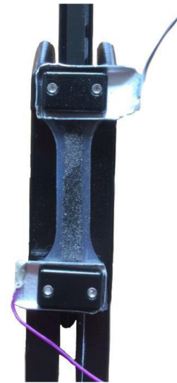
Figure 1 Stretchable Sensor attached to the Stretcher Machine
