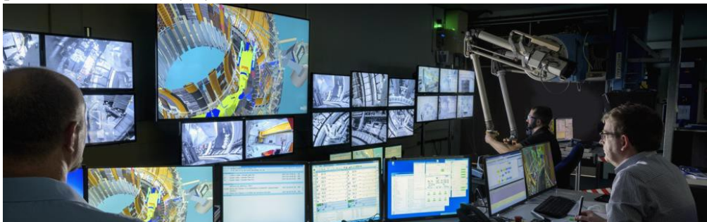
Figure 1: JET remote handling control room with SVS on central display.
