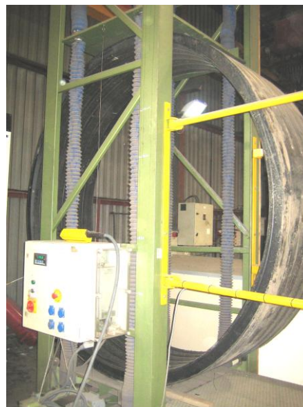
Fig. 2 A pipe sample placed in the pipe stiffness machine.
