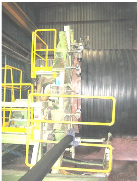
Fig. 1 The extruded profile is wound around the mandrel and welded to the adjacent one.
