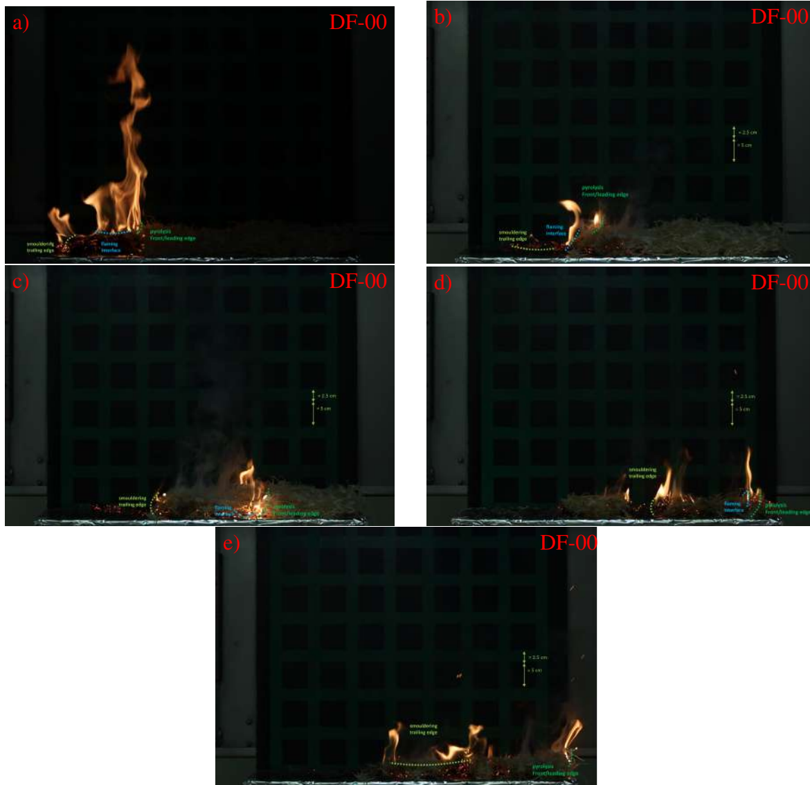
Figure 6.9: Flame heights at leading and trailing edges of fire for Excelsior fuel covered with plain dry foam (DF-00) at various positions across the fuel bed: a) leading edge at 20 cm, b) trailing edge at 20 cm, c) leading edge at 40 cm, d) trailing edge at 40 cm, and e) leading edge at 60 cm.
