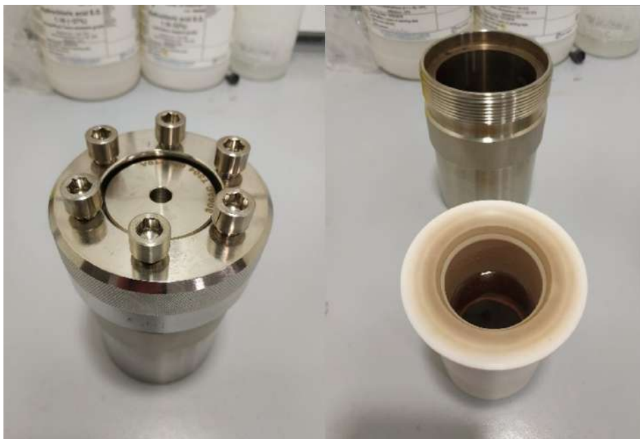
Figure 3.1: Stainless-steel pressure autoclave and a 125 mL Teflon liner used for Hydrothermal Synthesis.
