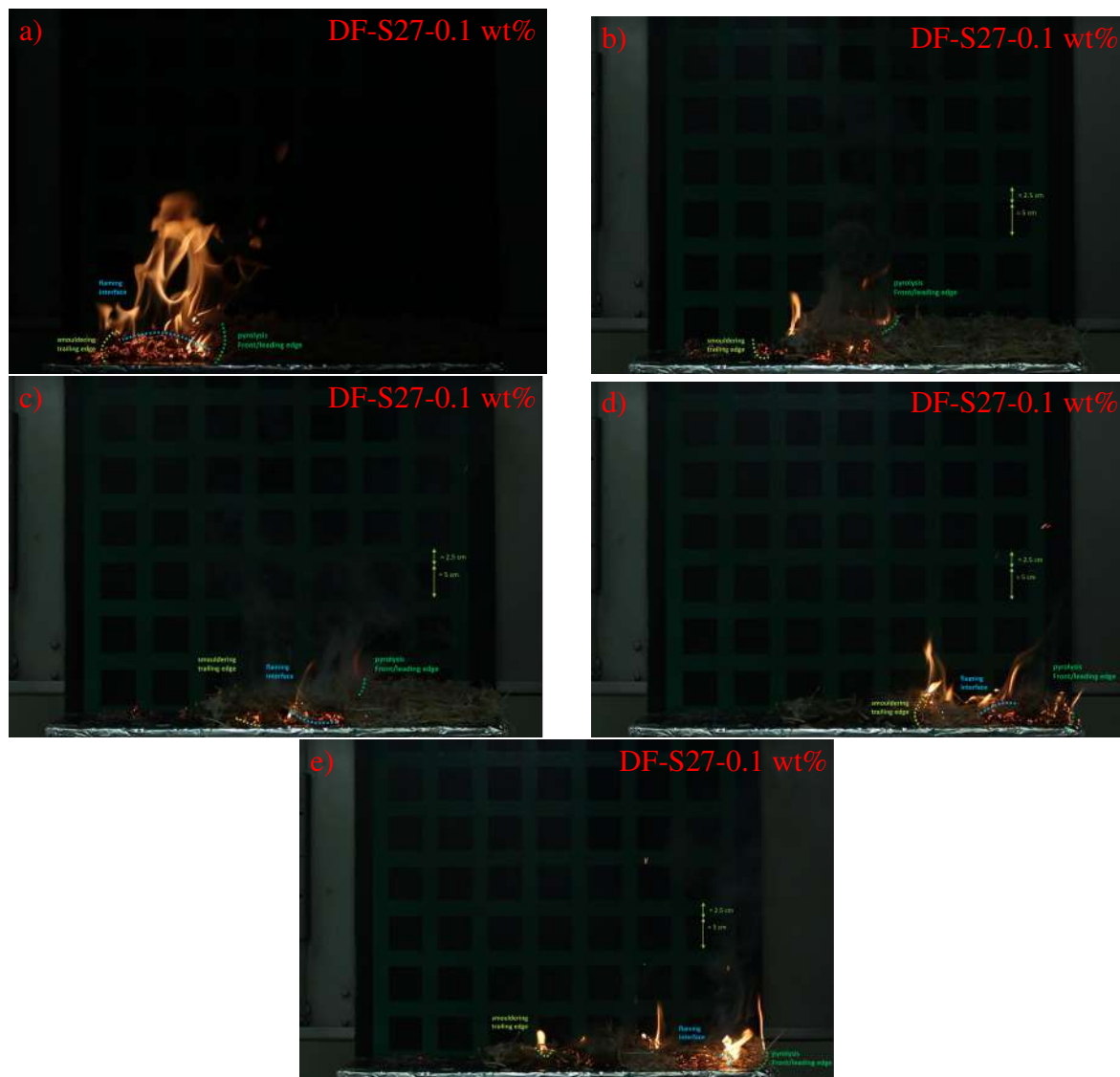
Figure 6.10: Flame heights at leading and trailing edges of fire for Excelsior fuel covered with dry foam and synthesised IONPs (DF-S27-0.1 wt%) at various positions across the fuel bed: a) leading edge at 20 cm, b) trailing edge at 20 cm, c) leading edge at 40 cm, d) trailing edge at 40 cm, and e) leading edge at 60 cm.
